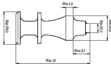
The stud dimensions for ice tyres mounted on a 7" x 15" rim are as follows:
